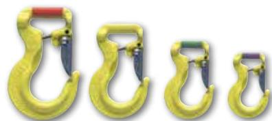
The roundsling hooks are colour coded in order to match the corresponding size of the roundsling: Red=5T / Yellow=3T / Green=2T / Violet=1T
