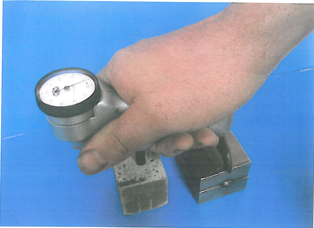
Figure 3.2: Use of a Barcol Hardness tester on a resin cube.
